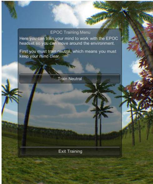
Before you can start to train any movements, you'll need to train the neutral action which is basically just keeping your mind clear of any thoughts. You need to do this first as the device needs to tell the difference between thinking of an action and not thinking of one.
